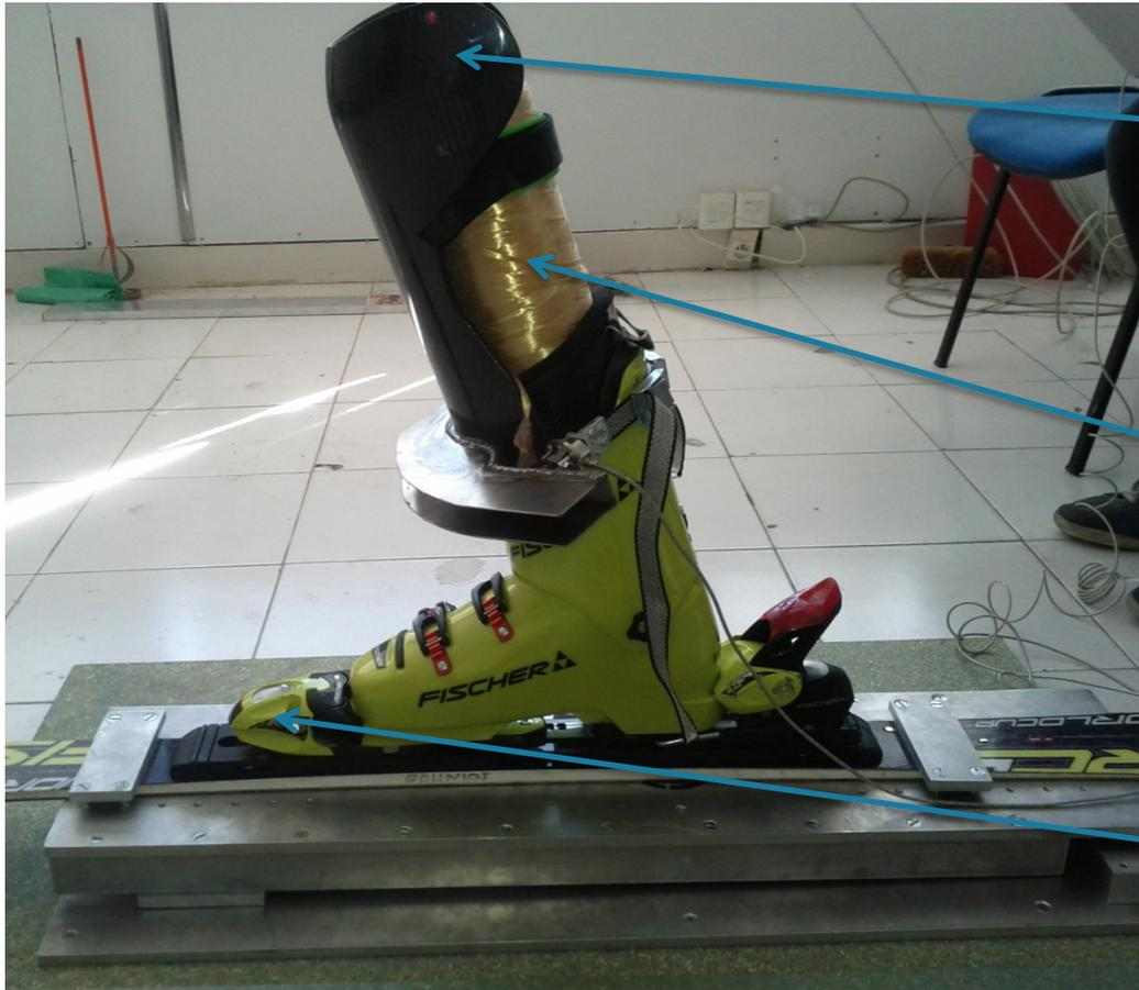
applying a manual force on the composite shell
